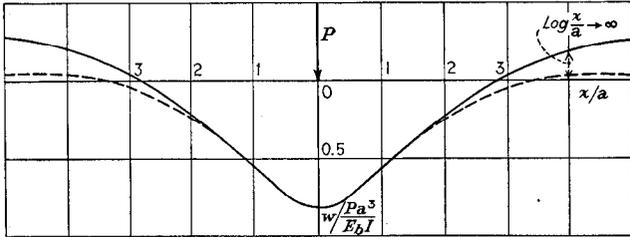
FIG. 5 DEFLECTION CURVES CORRESPONDING TO THE BENDING MOMENT CURVES OF FIG. 4
