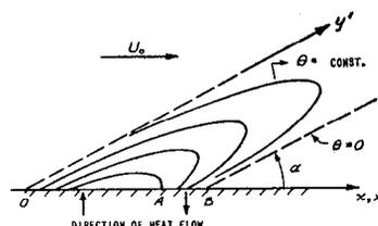
FIG. 3. Distortion of temperature field in the fluid due to its motion.
