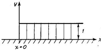
FIG. 6. Unit step temperature applied at the wall.
