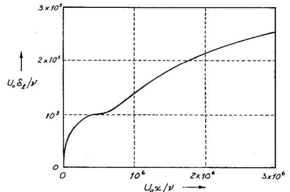
FIG. 9. Sublayer thickness  $\delta_l$  as a function of the distance  $x$  to the leading edge of a plate (Ref. 8).
