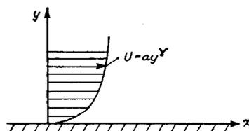
FIG. 7. Boundary layer with a power-law velocity profile.
