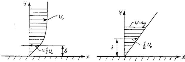
Fig. 4. (Left) Laminar boundary layer profile and displacement thickness  $\delta$ . FIG. 5. (Right) Linear velocity distribution.
