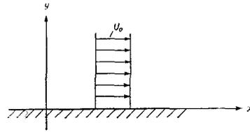
FIG. 1. Uniform flow near a wall.
