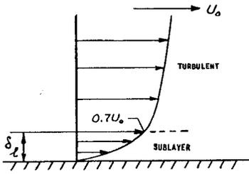
FIG. 8. Velocity profile of turbulent boundary layer on a flat plate. Thickness of the sublayer is  $\delta_l$ .
