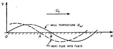
FIG. 2. Sinusoidal wall temperature  $\theta_w$  and the corresponding distribution of heat flux.
