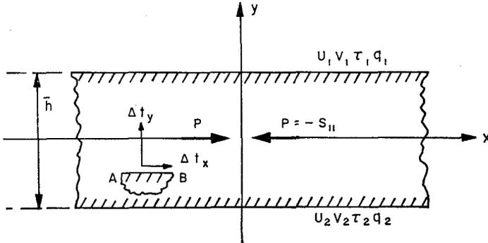
FIGURE 1. Plate under initial stress  $P$  viewed across the thickness.
