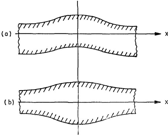
FIGURE 2. Antisymmetric (a) and symmetric (b) deformations of a plate.
