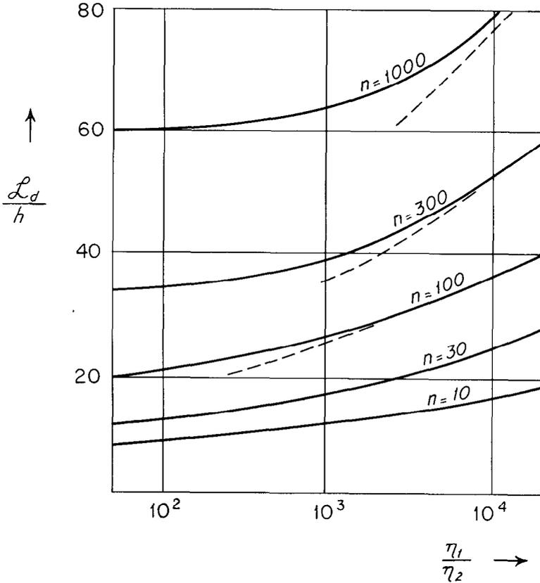
Figure 4. Wave length  $L_d$  of viscous buckling with all layers of equal thickness  $h$ . The number of confined layers is  $n = H/h$ , and the ratio of viscosities of two adjacent layers is  $\eta_1/\eta_2$ . Dashed curves represent equation 21.
