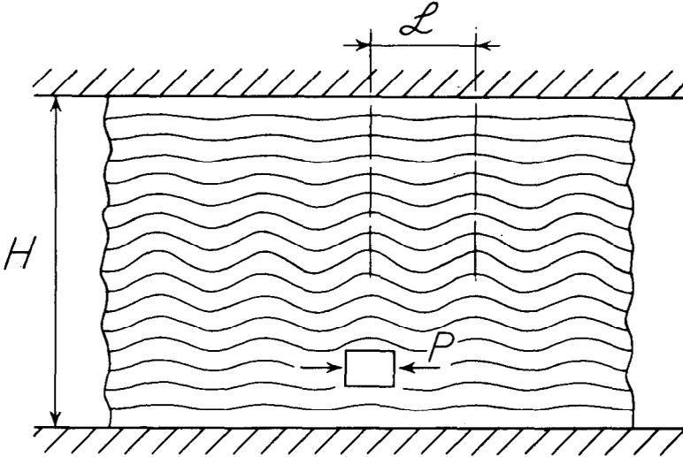
Figure 1. Internal buckling of a multilayered medium under rigid confinement
