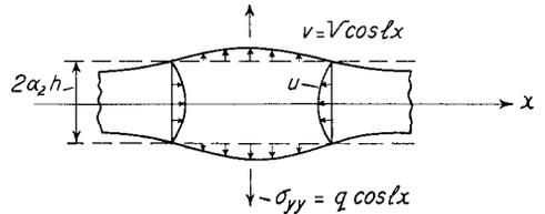
Figure 3. Deformation of the soft layer and associated interstitial flow represented by  $u$
