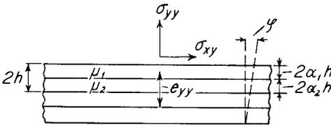
Figure 2. Details of multilayered structure and definition of the average coefficients  $L = \sigma_{xy}/\varphi$  and  $M = \sigma_{yy}/4\epsilon_{yy}$
