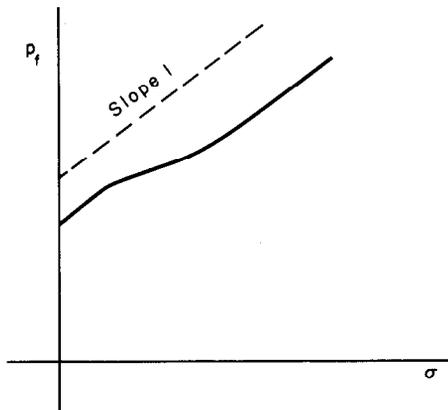
Fig. 8. Failure pressure  $p_f$  vs. hydrostatic stress  $\sigma$  for non-linearity illustrated in Fig. 6.
