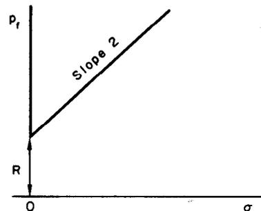
Fig. 2. Failure pressure  $p_f$  vs. hydrostatic stress  $\sigma$  for linear material.
