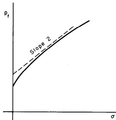
Fig. 5. Failure pressure  $p_f$  vs. hydrostatic stress  $\sigma$  for non-linearity illustrated in Fig. 3.
