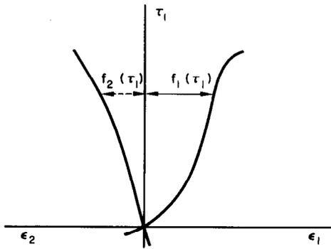
Fig. 3. Stress-strain functions corresponding to one type of non-linearity.
