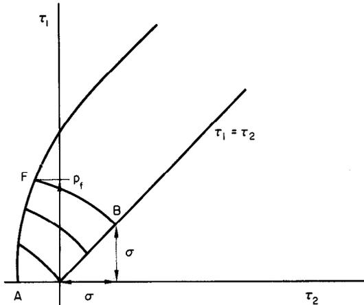
Fig. 7. Diagram  $\tau_1, \tau_2$  for non-linearity illustrated in Fig. 6.
