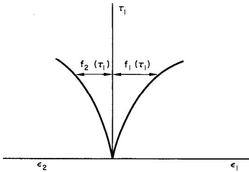
Fig. 6. Stress-strain functions corresponding to another type of non-linearity.
